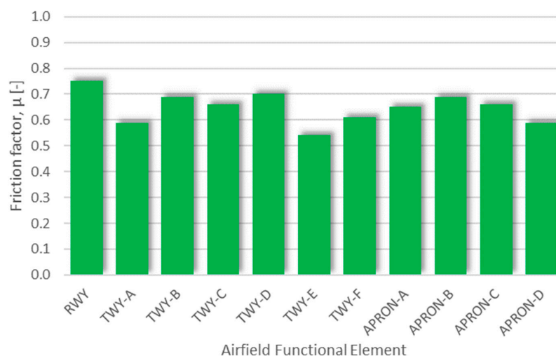
Figure 11. Test results for pavement anti-skid properties.
