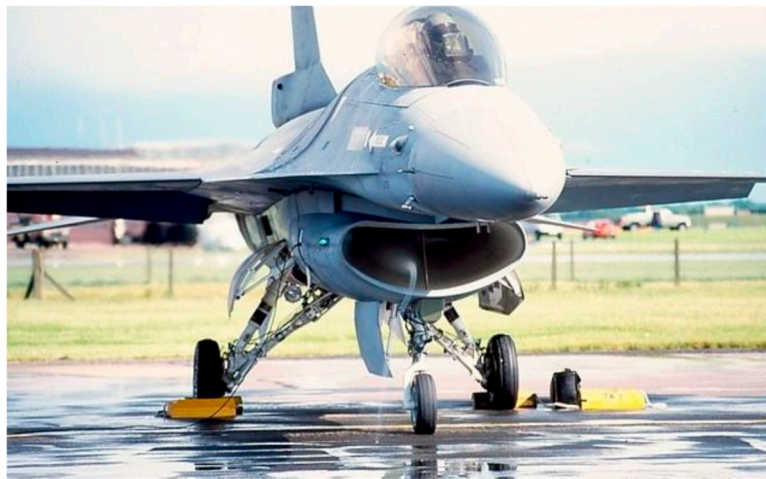
Figure 1. Water whirlpool being created as the result of air sucked in by the jet engine. Source: [4].
